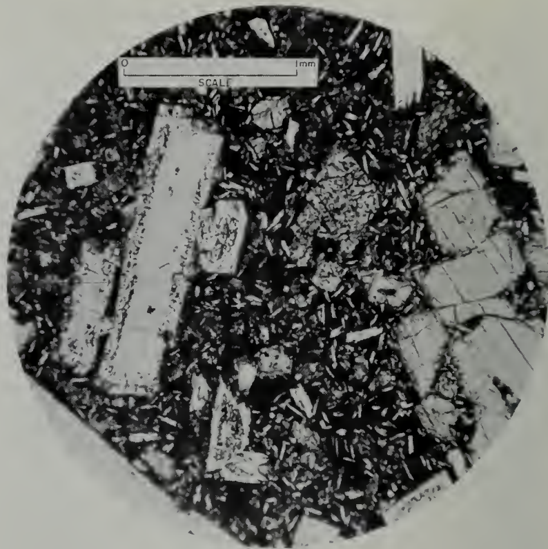
Photo 9. Basalt, Plush Ronch member four, showing vermicular tubules of glass in lobradorite (left) and ougite and hypersthene (right). Crossed nicols.
